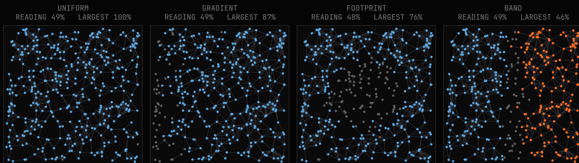
FIGURE 2 One realisation of each of four scenarios on the same formation, all with a dashboard reading near 50%. Units in the largest connected group are blue, units in a second large group are orange, and units in small fragments are grey. Working links are drawn in dark grey. From left to right, failures are spread uniformly, arranged in a gradient from right to left, concentrated in a footprint in the middle, and concentrated in a band down the middle.
